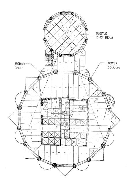
Figure 1 Typical Floor below level 38 (Petronas Twin Tower Project)
