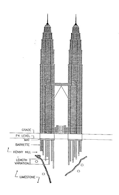
Figure 2 Elevation including foundation details (Petronas Twin Tower Project)
